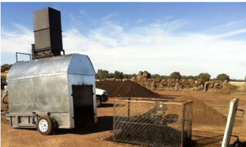
Figure 3.6 The Big Roo 4 cum portable batch kiln designed for straw. ( www.allthingsbiochar.com.au for further information)
