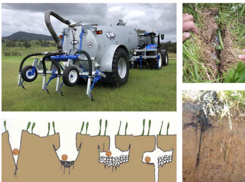
Figure 8.4 Top left: Subsoil injection equipment. 6 Bottom Left: different shaped seed and slurry cavities in soil made by (from left) double-disk seed drill, hoe seed drill, Baker Boot seed drill, and combined winged tine and disk. Right: Views from above and in soil profile showing biochar slurry occupying both the horizontal seed bed shelves, and the vertical disk cut. (Graves 5 )
