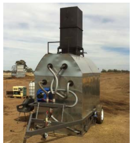
Figure 3.6 The Big Roo 4 cum portable batch kiln designed for straw. ( www.allthingsbiochar.com.au for further information)
