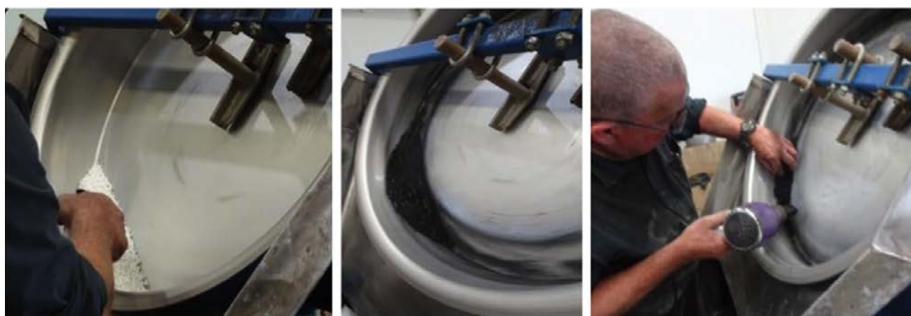
Figure 7.14 Coating urea granules. Left: Adding a mixture of damp clay and biochar powder to urea granules in a plate agglomerator. Middle: The clay and biochar are coating the urea granules. Right: Drying the granules with a hair dryer
