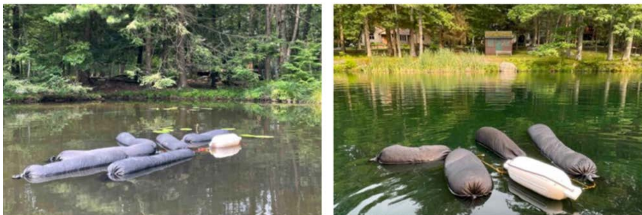
Figure 7.8 Left: Biochar-filled bags in a nutrient-loaded pond. Right: Biochar-filled bags have adsorbed nutrients from the pond water, resulting in a clean-water pond. 19
