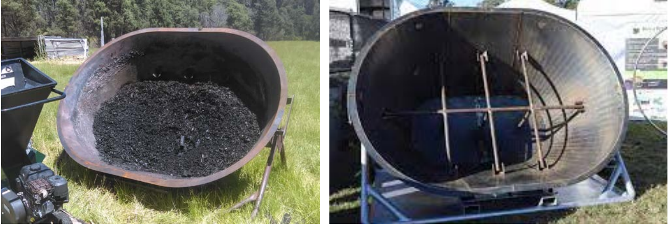
Figure 3.7 Commercial stretch Kon-Tiki Kiln, produced by Terra Preta Developments Pty, Ltd.
