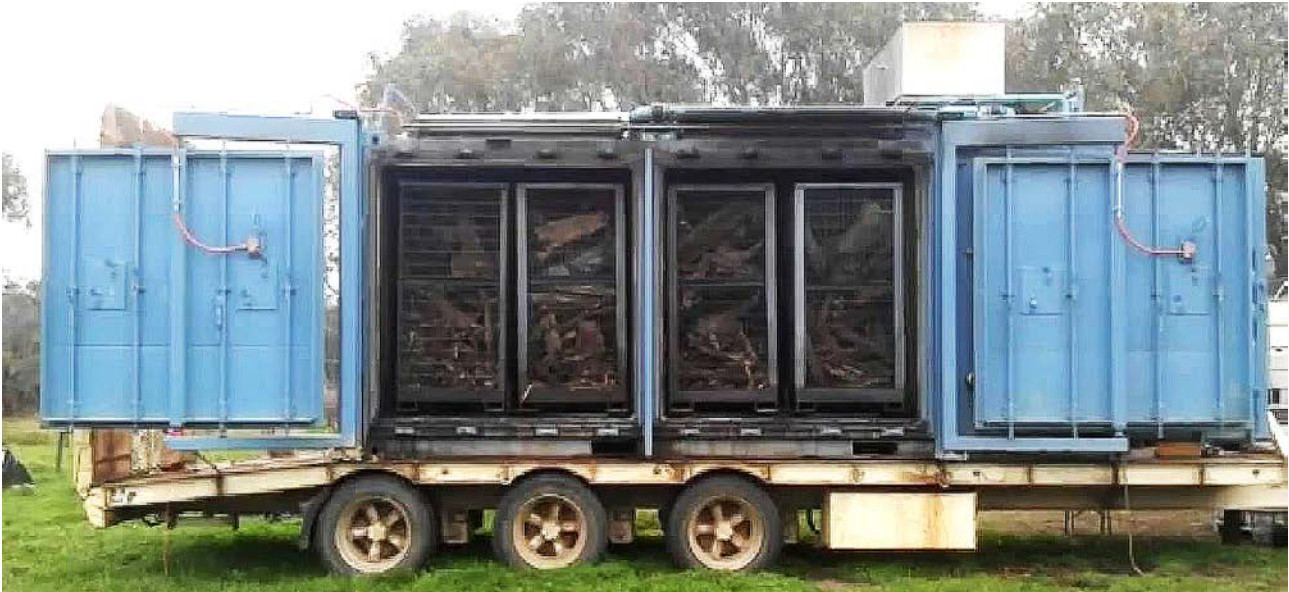
Figure 3.5 Earth Systems batch kiln. www.esenergy.com.au/charmaker-2 for further information
