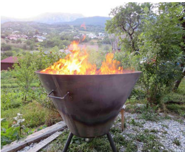
Figure 3.1 Left: The original 1.5 m diameter deep cone Kon-Tiki, developed at Ithaka Institute in Switzerland. The flame cap burns gases cleanly and protects the char from oxygen. Right: Convection dynamics of the Kon-Tiki. Updraft past the rim of the kiln entrains a rolling vortex inside the kiln. This pulls air down into the centre of the kiln, providing primary air for pyrolysis. Gases and smoke released from the pyrolysis zone are captured into the vortex and become mixed with air in the flame zone for cleaner combustion. A heat shield (optional) enclosing the kiln strengthens the natural vortex dynamic of the Kon-Tiki and makes the kiln more comfortable and efficient to operate. (Photo: Paul Taylor, Hans Peter Schmidt.)
