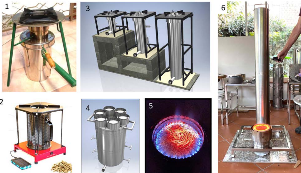
Figure 3.3 Biochar-making gasifier cook stoves. 1. Champion TLUD Stove developed by Paul Anderson and manufactured by Servals in India. 2. FabStove, a fan driven advance on the Champion manufactured in South Africa and available online. 3–6. A range of gasifiers developed and photo'd by Paul Olivier in Vietnam: 3. Household stoves 250, 500, and 800 mm tall. 4. 800 mm tall, 500 mm diameter, 80 kW gasifier with multiple burners. 5. Nichrome wire burner on gasifier running on mesquite pellets. 6. 1200 mm tall bottom-lit downdraft gasifier with a run time of 8 hours
